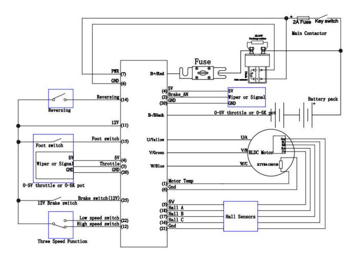
**Figure 7: KLS-S** controller standard wiring(Three speed function control) (Battery voltage can be used for controller supply)
