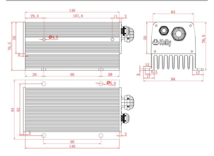
Figure 2:KLS6018S mounting holes' dimensions (dimensions in millimeters)
