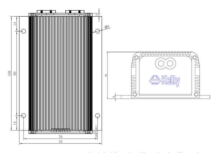
Figure 1:KLS4812S KLS7212S mounting holes' dimensions (dimensions in millimeters)
