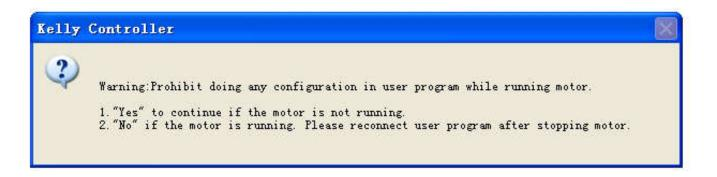
Anyway please try to do identification angle operation before running the motor. And please don't try to connect the controller to user program while the motor is still running,let alone change the setting in user program or Android App.That is to say,if you want to connect controller to user program or try to do programming,please stop the motor first.
