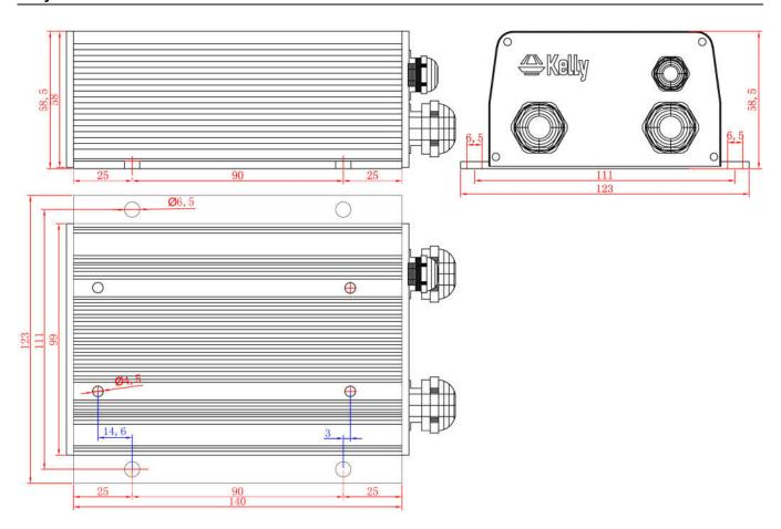
Figure 4:KLS6030S KLS6035S KLS7230S mounting holes' dimensions (dimensions in millimeters)
