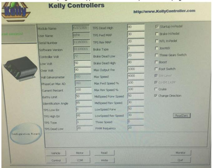
Please check whether the Identification Angle item is at 85 or not. It is correct if identification angle item is at 85. But customers still need to run identification angle operation before driving. Because the 85 means this controller finished the identification angle operation with the motor in factory before shipment. Your motor is different from the motor from controller supplier.
