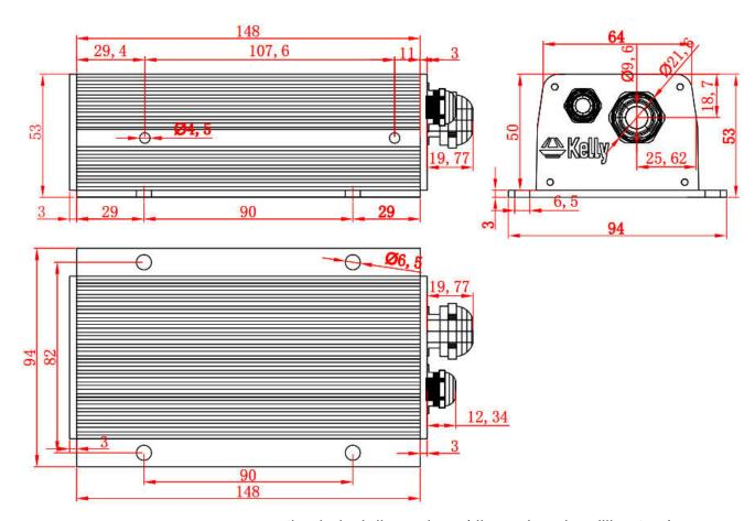
Figure 3:KLS7218S mounting holes' dimensions (dimensions in millimeters)
