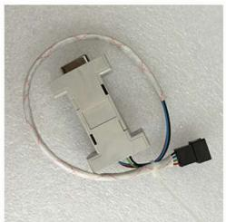
Customers also can use a Z-TEK USB to RS232 cable and SM-4A DB9(RS232) Converter to connect the controller to an Android Tablet.
