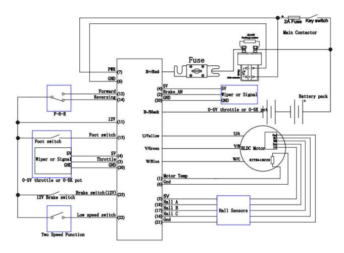
**Figure 6: KLS-S** controller standard wiring(F-N-R control) (Battery voltage can be used for controller supply)
